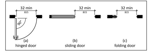
Accessible doors should provide at least 32 inches of clear width. Clear width is measured between the face of the door itself and the opposite stop.
