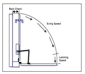
The closing or swing speed must not be faster than five seconds. The closing or swing distance is from the open position at 90 degrees to 12 degrees from the latch. Latching speed isn't specified, but should be fast enough to latch the door but not slam it.
