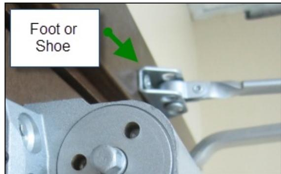
the hinge side of the door, increasing the power up to 15%. With a closer with a three-hole shoe, you can increase the power up to 7.5% by moving the arm from the center position to the hinge side of the door. Moving the arm from the center position to the latch side of the door can decrease the power as much as 7.5%.
