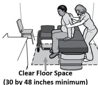
**Provide a minimum clear floor space of 30" x 48" next to exam tables, so that individuals can transfer easily onto the tables.**
