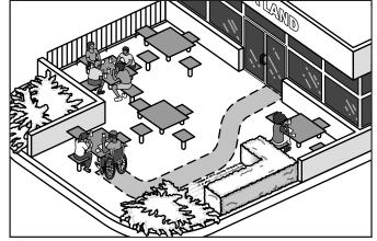
Accessible table: table-top surface should be no higher than 34 inches above the floor and clear space underneath at least 27 inches high (for wheelchair users to get their feet and knees under the table).
