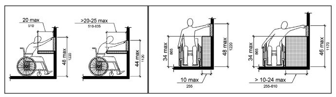
Image note: Reach range is listed first in inches and then in centimeters.
