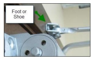
the hinge side of the door, increasing the power up to 15%. With a closer with a three-hole shoe, you can increase the power up to 7.5% by moving the arm from the center position to the hinge side of the door. Moving the arm from the center position to the latch side of the door can decrease the power as much as 7.5%.
