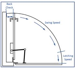
• The closing, or swing speed must not be faster than five seconds. The closing or swing distance is from the open position at 90 degrees to 12 degrees from the latch. Latching speed isn't specified, but should be fast enough to latch the door but not slam it.
