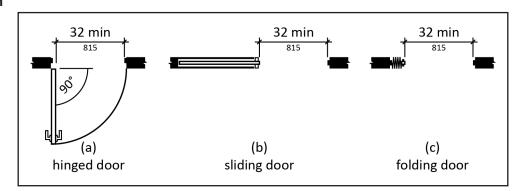
Accessible doors should provide at least 32 inches of clear width. Clear width is measured between the face of the door itself and the opposite stop.
